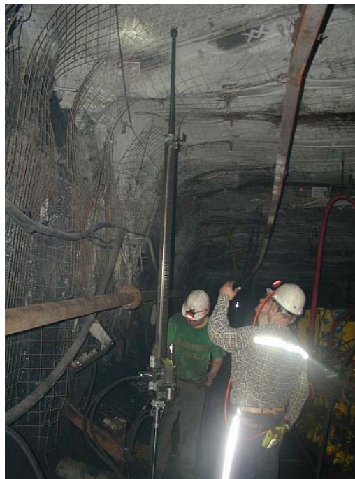
Photo of the drill VS 1 WK during the testing operation under mine underground conditions
