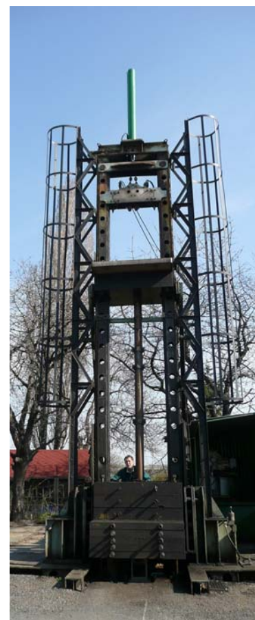
Fig. 2 – Mechanical strut located in the fall stand after the dynamical test
