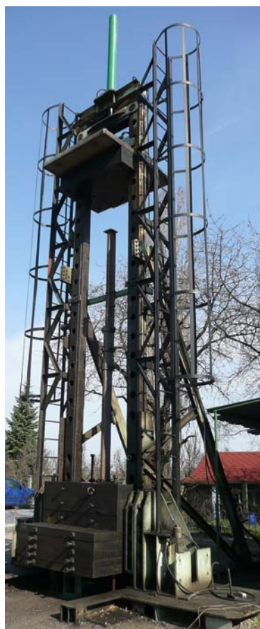
Fig. 1 – Mechanical strut located in the fall stand before dynamical test
